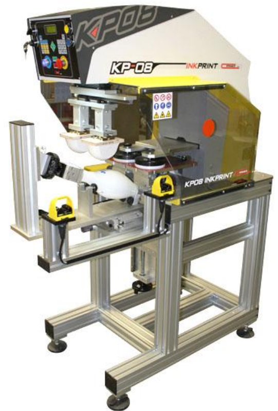
Figure 1: A standard KP08 with a programmable custom fixture. The part rotates and the pads shuttle to print separate images on both sides. Safety features include thumb switches to ensure operator is clear of any moving part during the print cycle.
